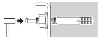
6) Tighten the nut with a spanner to secure the wall plate to the wall.
